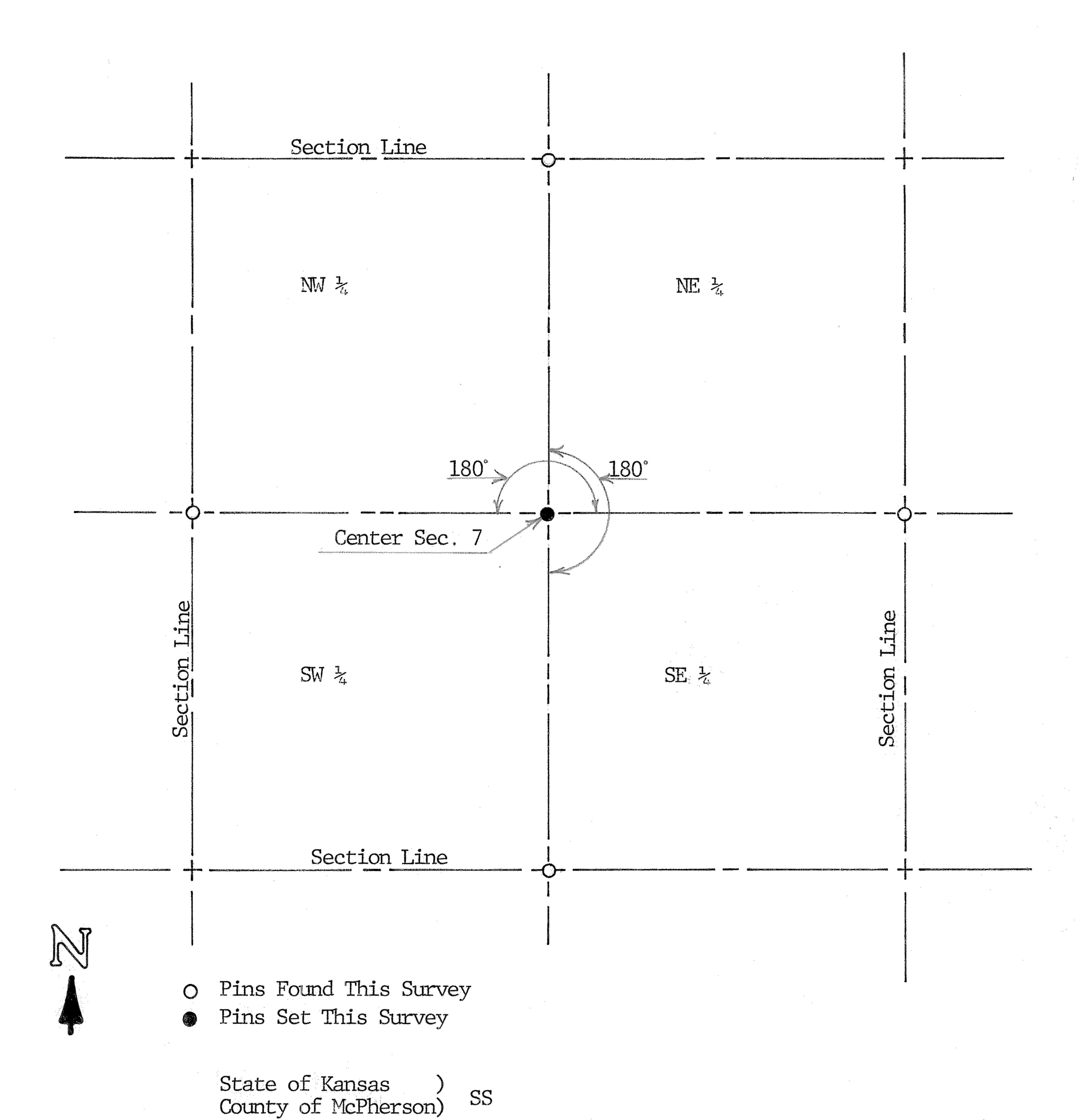
I, Melvin Ferguson, County Engineer of McPherson County, do hereby certify that under my supervision a survey was made to establish the center of Section 7, T21S, R4W of the 6th P.M.
