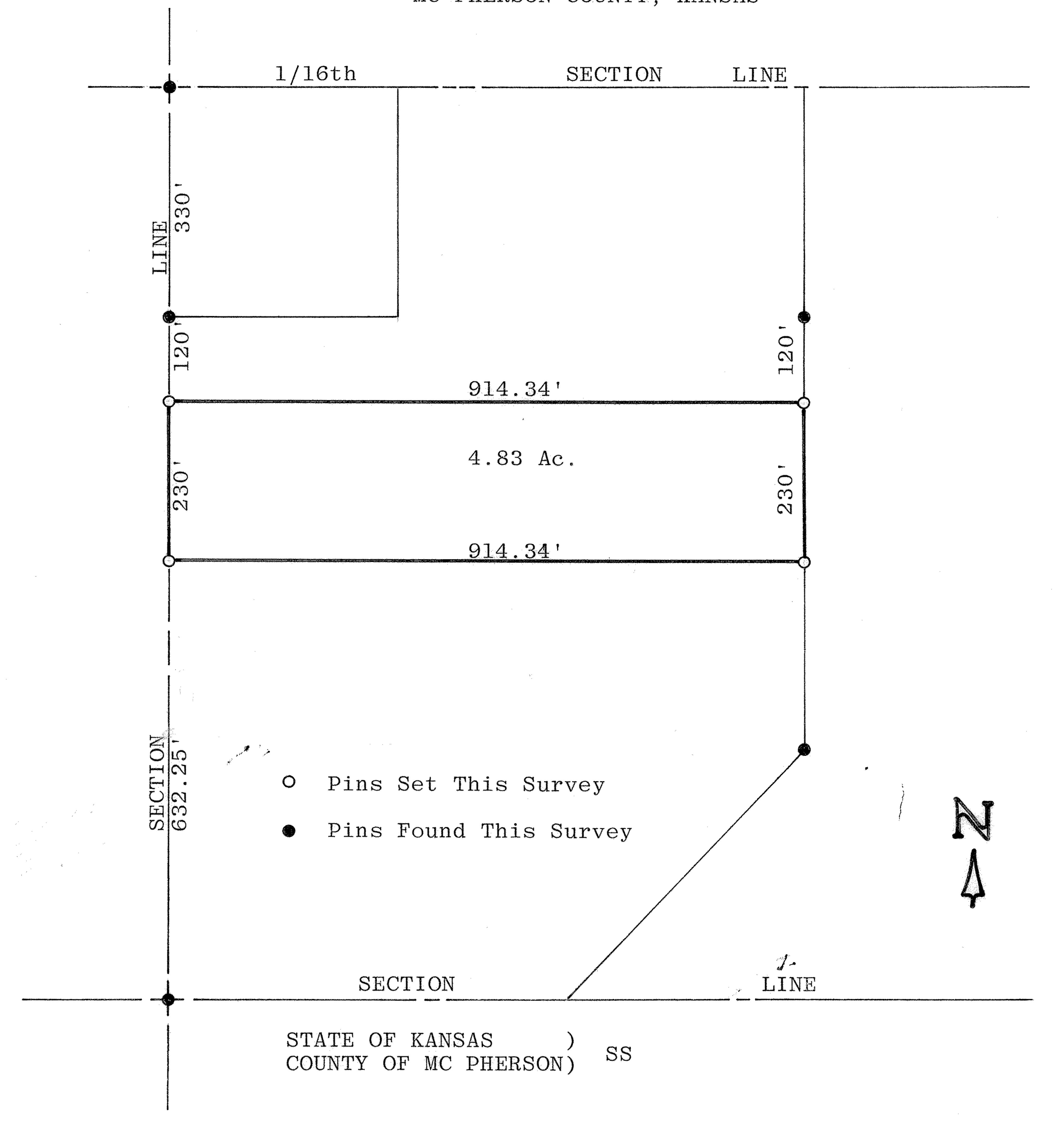
I, Melvin Ferguson, County Engineer of McPherson County, Kansas, do hereby certify that under my supervision a survey was made of a tract of land in the  $SW\frac{1}{4}$ ,  $SW\frac{1}{4}$  of Section 34, Tl9S, R3W of the 6th P.M. and described as follows:
