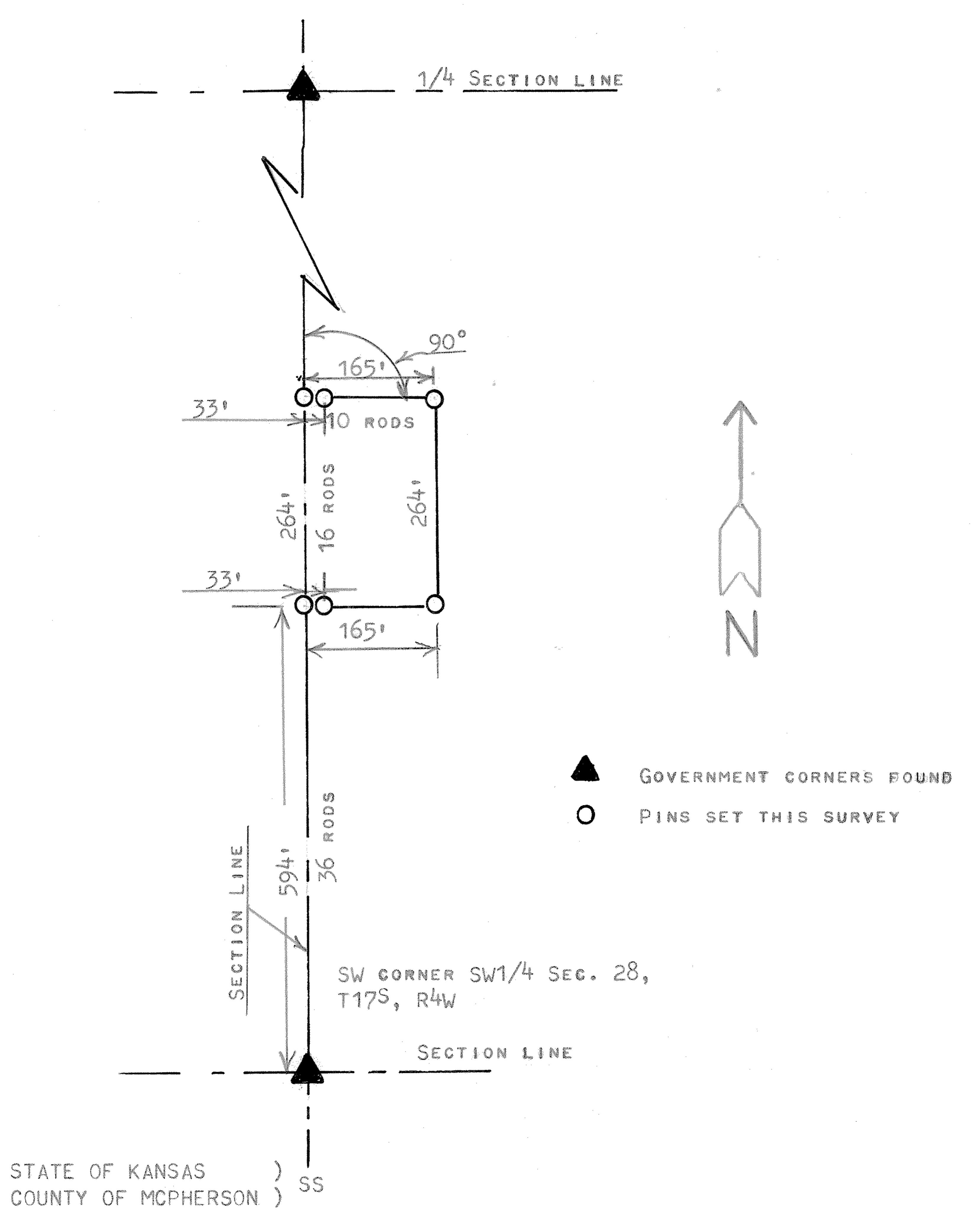
1, MELVIN FERGUSON, PROFESSIONAL ENGINEER OF THE STATE OF KANSAS DO HEREBY CERTIFY THAT UNDER MY SUPERVISION A SURVEY WAS MADE OF A TRACT OF LAND IN THE SW1/4, SECTION 28, T17S R4W OF THE 6TH P.M. AND DESCRIBED AS FOLLOWS:
