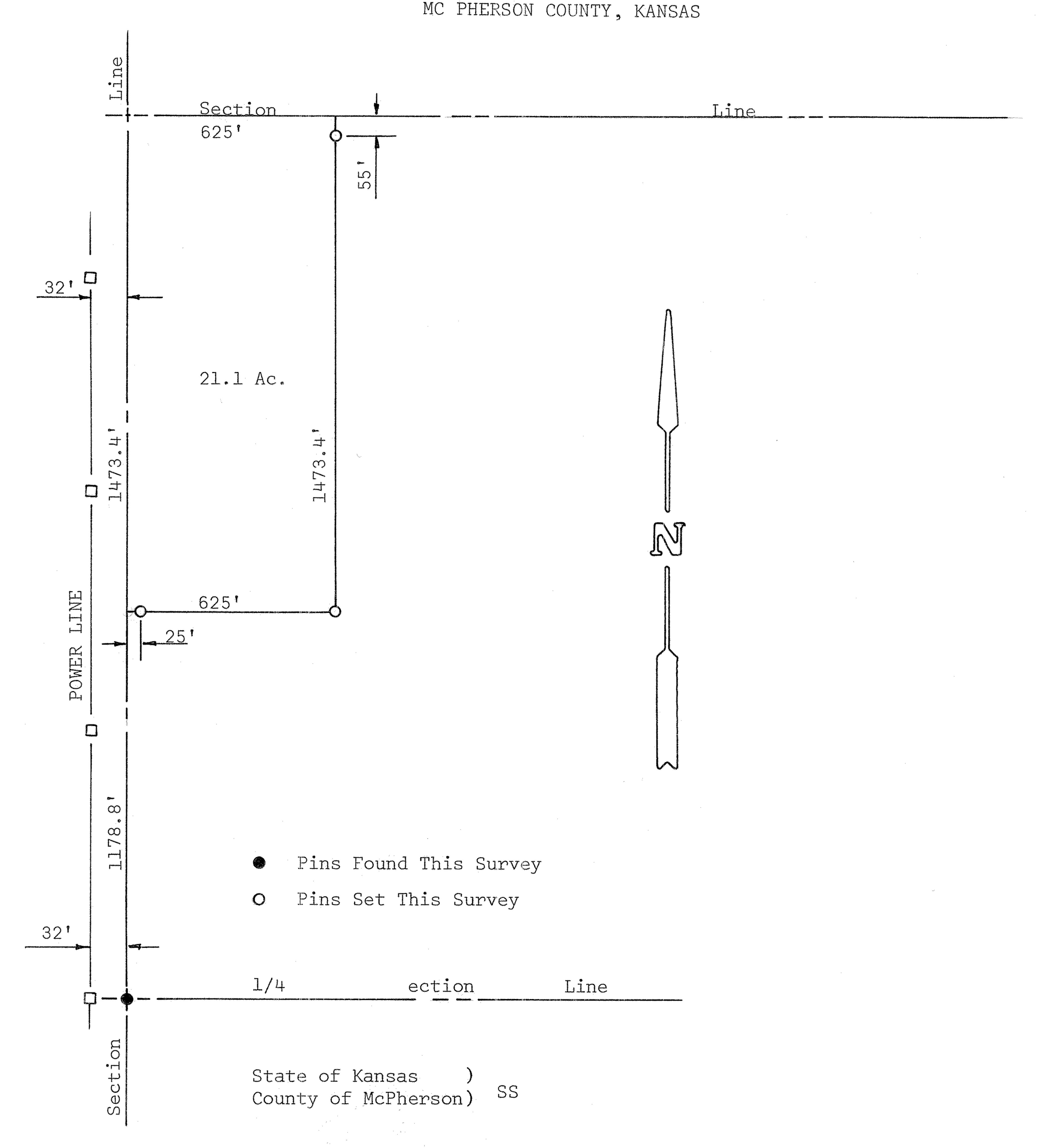
I, Melvin Ferguson, County Engineer of McPherson County, Kansas, do hereby certify that under my supervision a survey was made of a tract of land in the NW4 of Section 26, T21, R4W of the 6th P.M. and described as follows:
