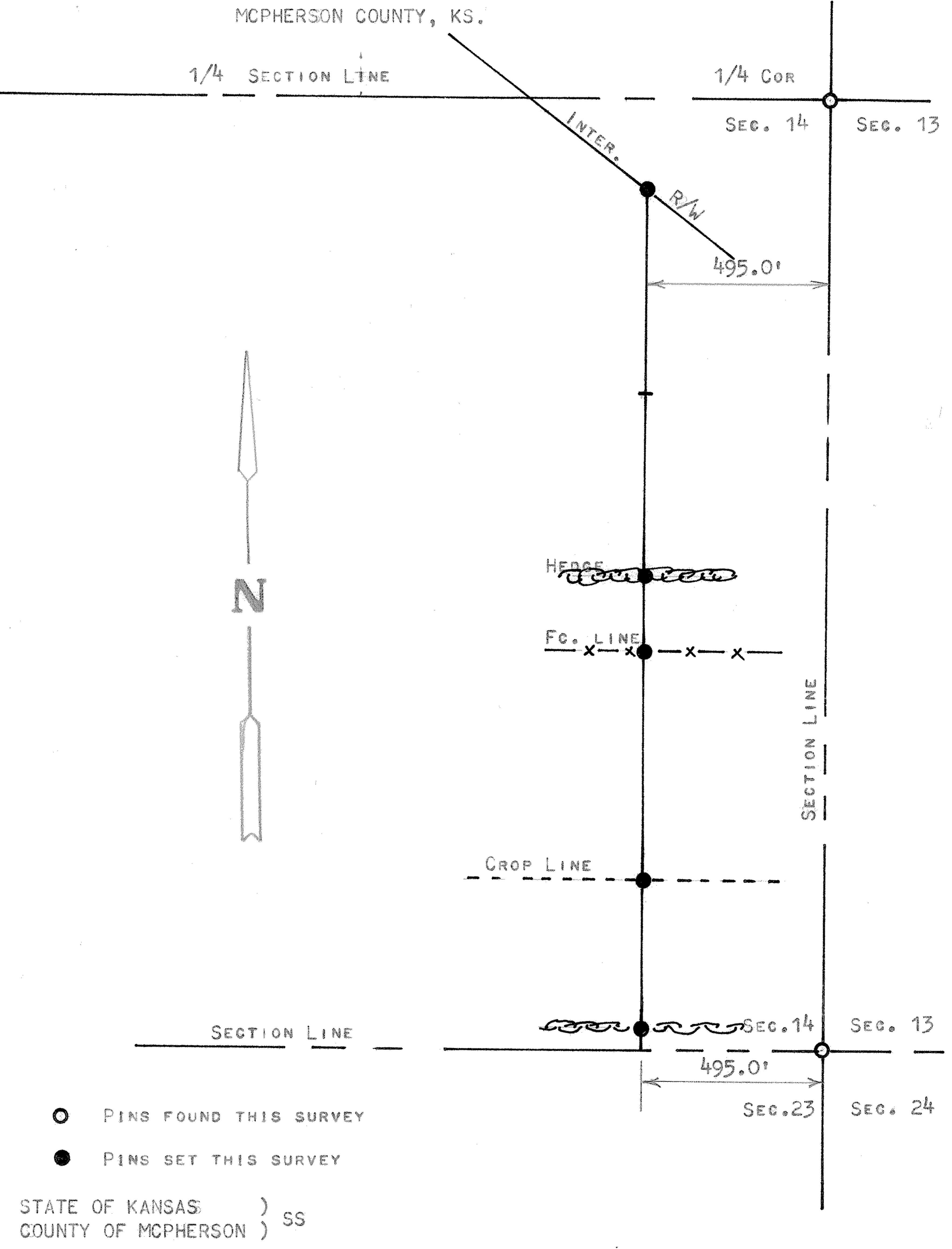
I, FRANCIS RANKIN, PROFESSIONAL ENGINEER OF THE STATE OF KANSASS DO HEREBY CERTIFY THAT UNDER MY SUPERVISION A SURVEY WAS MADE TO DETERMINE A LINE 495.0 FEET WEST OF THE EAST SECTION LINE IN THE SE 1/4, SECTION 14, T20S R3W OF THE 6TH P.M. AND THAT THE ACCOMPANYING PLAT IS A TRUE EXHIBIT OF SAID SURVEY AS FAR AS IT IS KNOWN TO ME.
