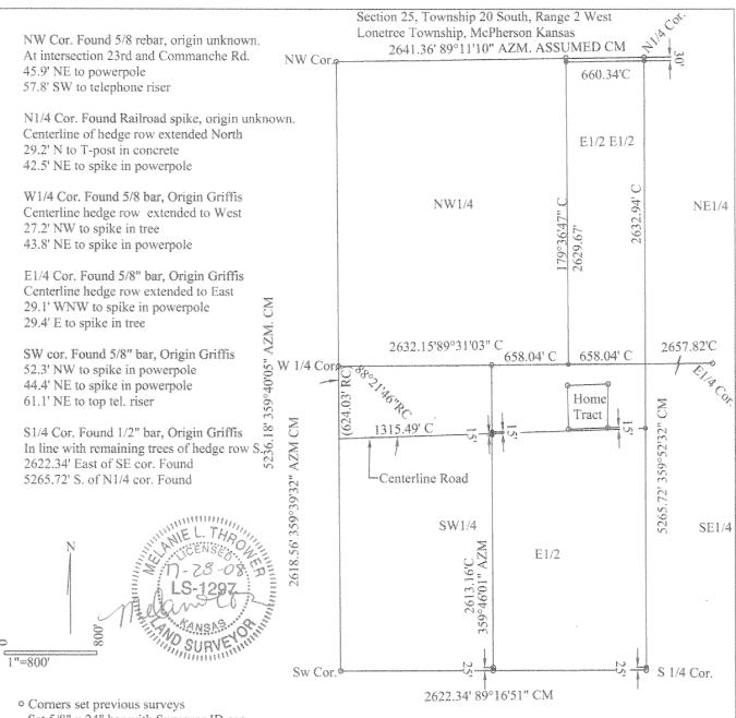
Set 5/8" x 24" bar with Surveyor ID cap (Note- 5' Green and White Metal T post with flagging was set at all corners this survey at off road boundary locations per client request)
