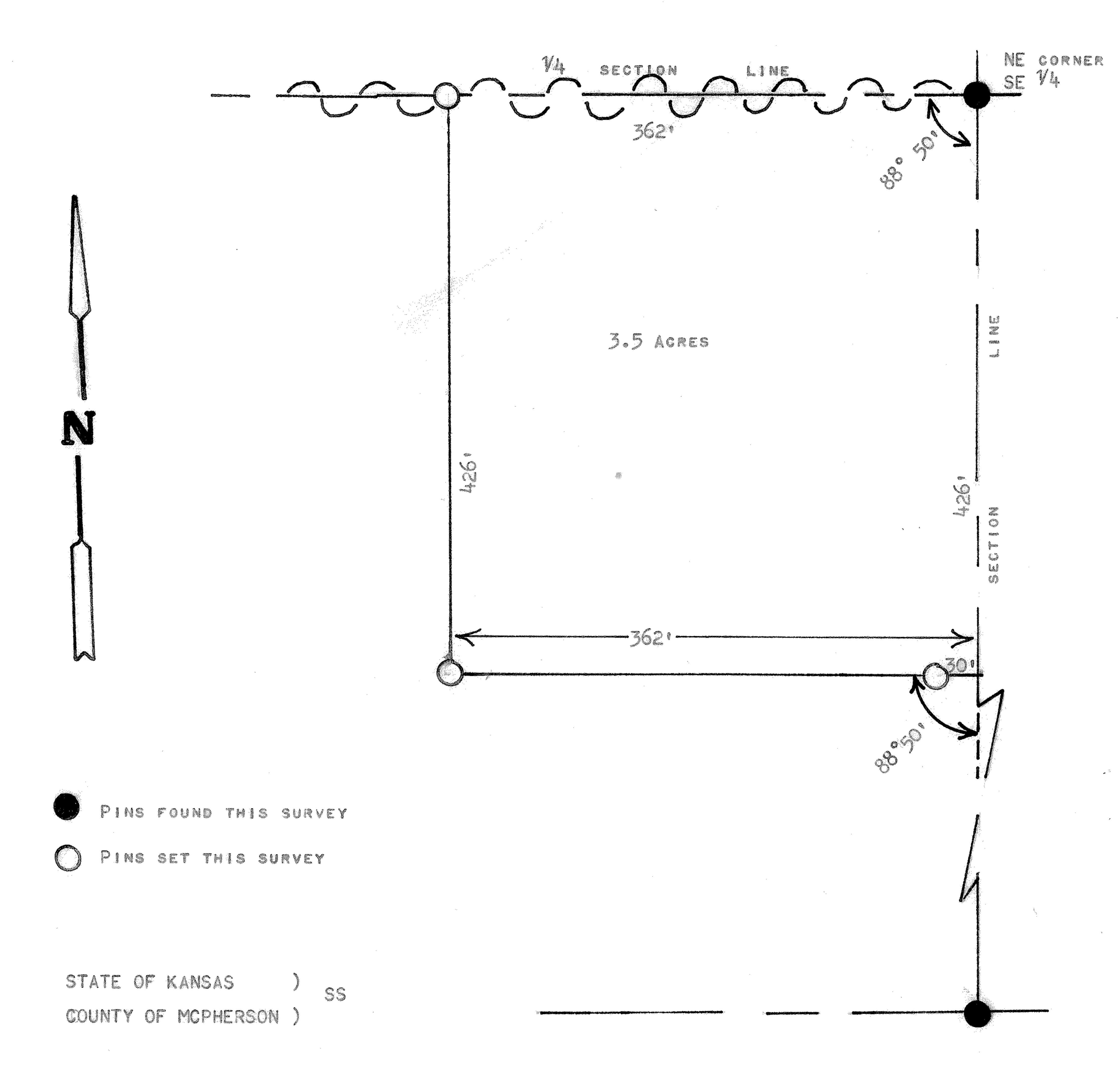
I. FRANCIS RANKIN, COUNTY ENGINEER OF MCPHERSON COUNTY, KANSAS, DO HEREBY CERTIFY THAT UNDER MY SUPERVISION A SURVEY WAS MADE OF A TRACT OF LAND IN THE SE 14 OF SECTION 1, T20S-R2W OF THE 6TH P.M. AND DESCRIBED AS FOLLOWS:
