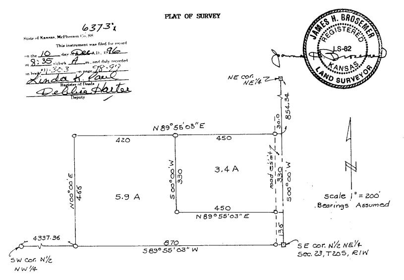
Legend:  $0=\frac{1}{2}$  rebar with ID cap (set)  $\Pi = \frac{5}{8}$  rebar (found)
