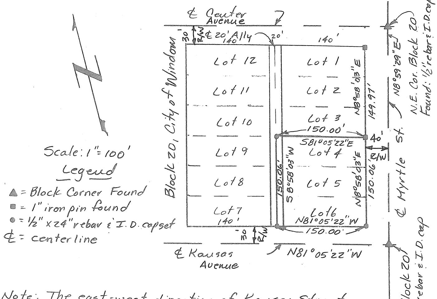
Note: The east-west direction of Kansas Street was determined by using property pins found on the south side of Lot 11 in Blk 41 in The City of Windom. I found  $\frac{1}{2}$ " rebars in concrete at the SE & SW corners of said Lot 11.
