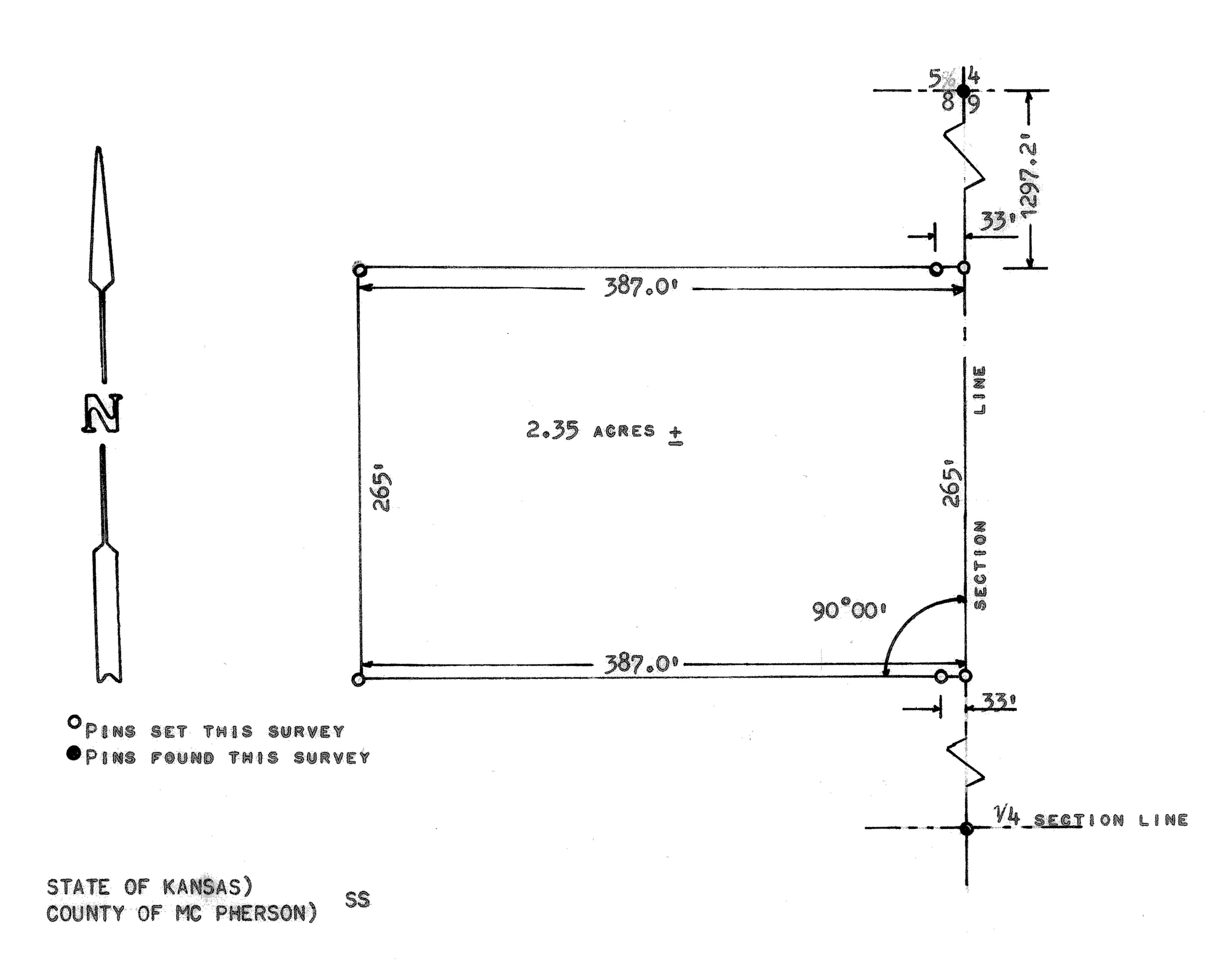
I, Melvin Ferguson, County Engineer of McPherson, Kansas do hereby gertify that under my supervision a survey was made of a tract of land in the NE  $^{74}$ , Section 8, T19S-R3W of the 6th P.M., and described as follows:
