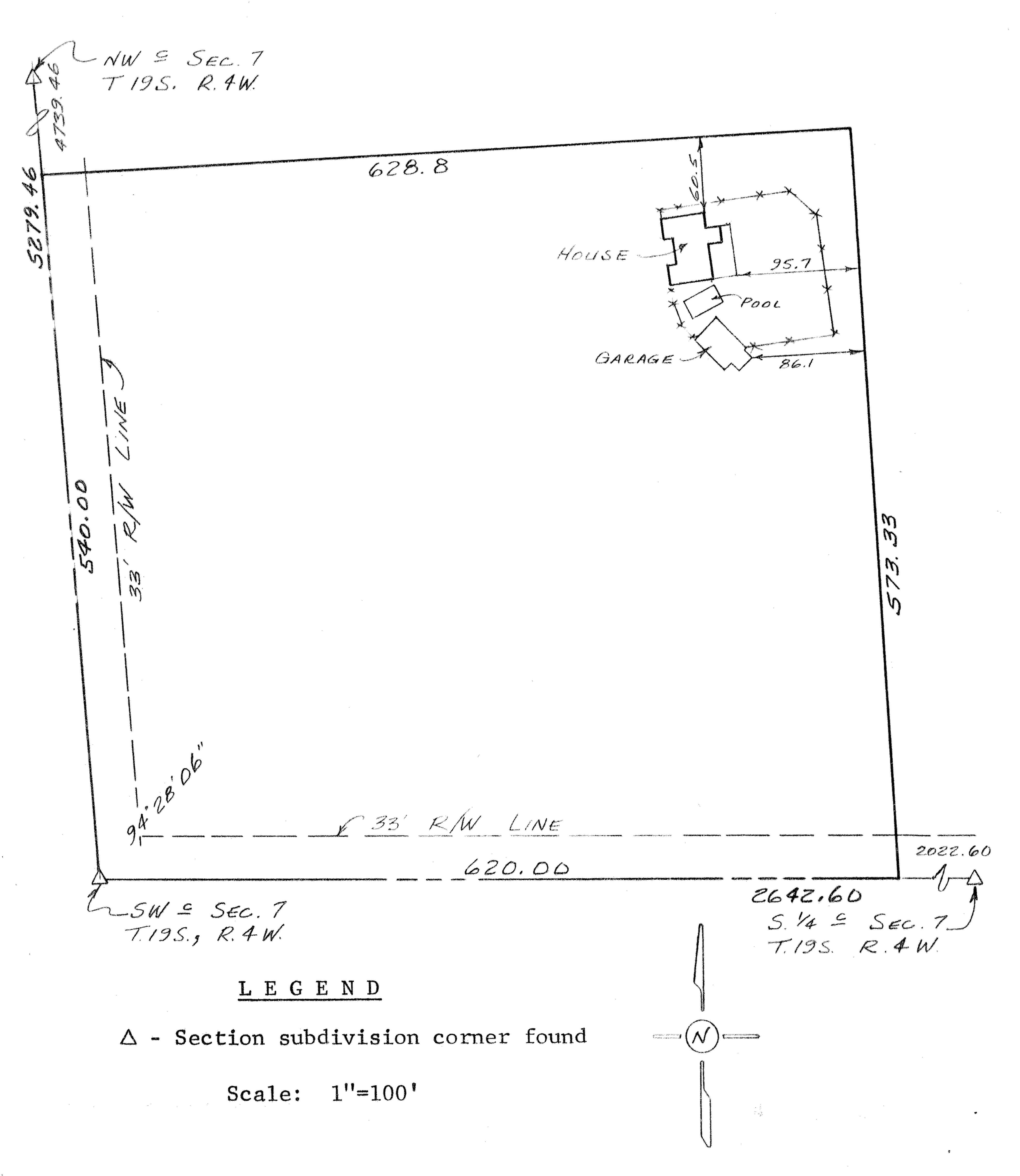
I hereby certify this plat to be a true, correct and complete representation of the property described above and on the attached sheet and the improvements located thereon and that there are no encroachments or overlaps either way across property lines, as surveyed by me, this 6th day of June, 1984.
