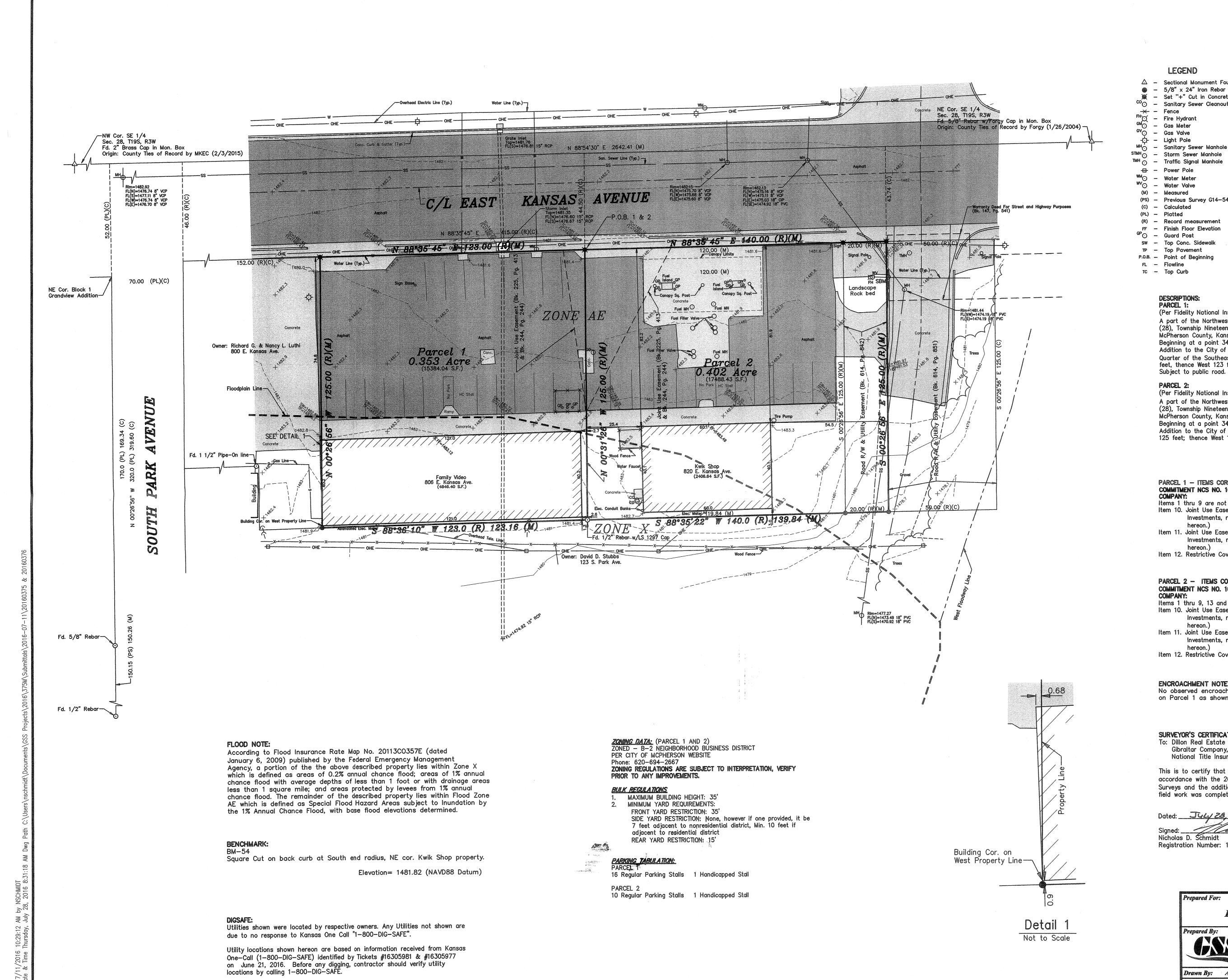
△ - Sectional Monument Found — 5/8" x 24" Iron Rebar Set w/G.S.S. Cap <sup>co</sup>⊙ — Sanitary Sewer Cleanout (PS) - Previous Survey G14-544 8/8/2014 BASIS OF BEARING = NAD 83 KANSAS SOUTH ZONE
