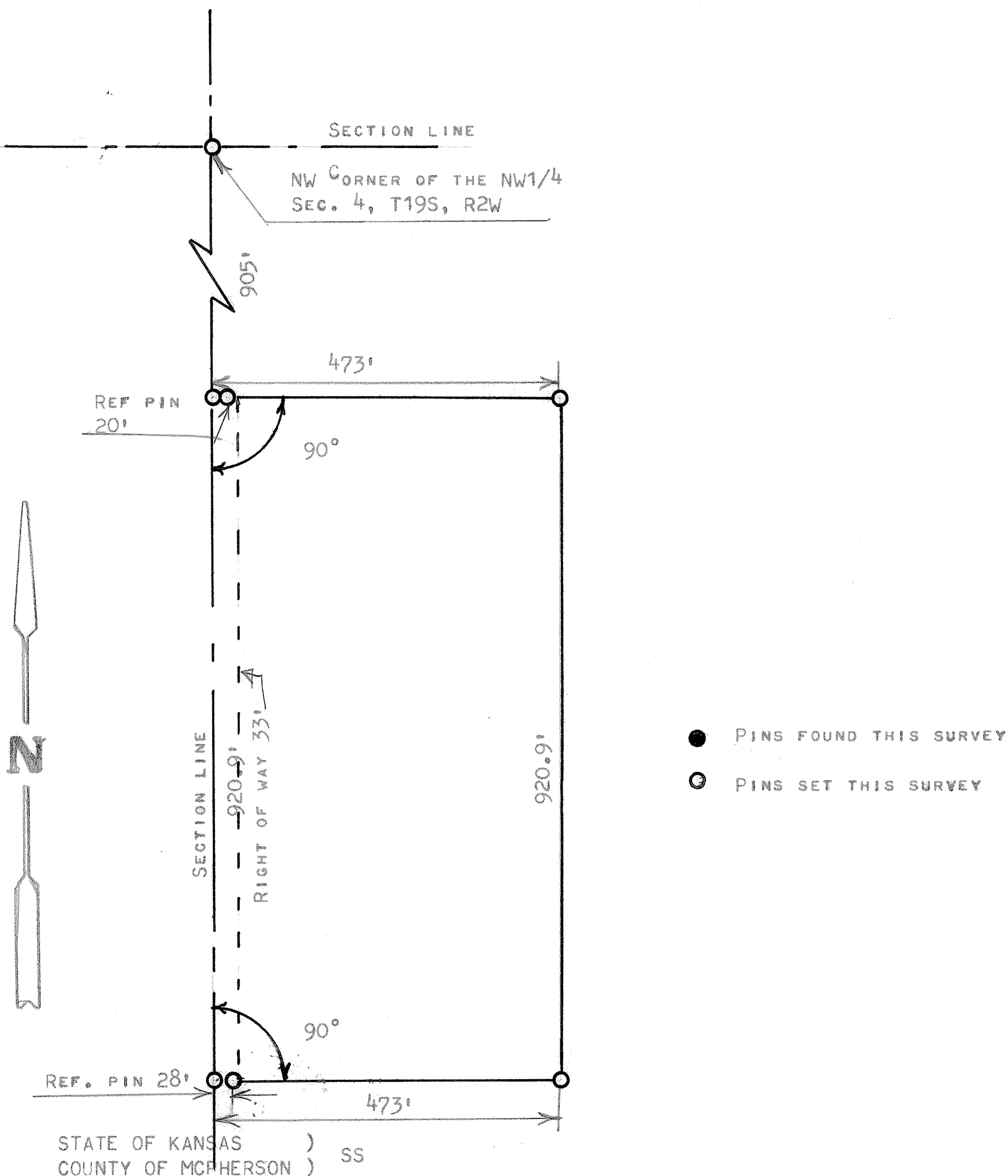
I, MELVIN FERGUSON, PROFESSIONAL ENGINEER OF THE STATE OF KANSAS DO HEREBY CERTIFY THAT UNDER MY SUPERVISION A SURVEY WAS MADE IN THE NW $\frac{1}{4}$ , SECTION 4, T19S, R2W OF THE 6TH PM.M AND DESCRIBED AS FOLLOWS;
