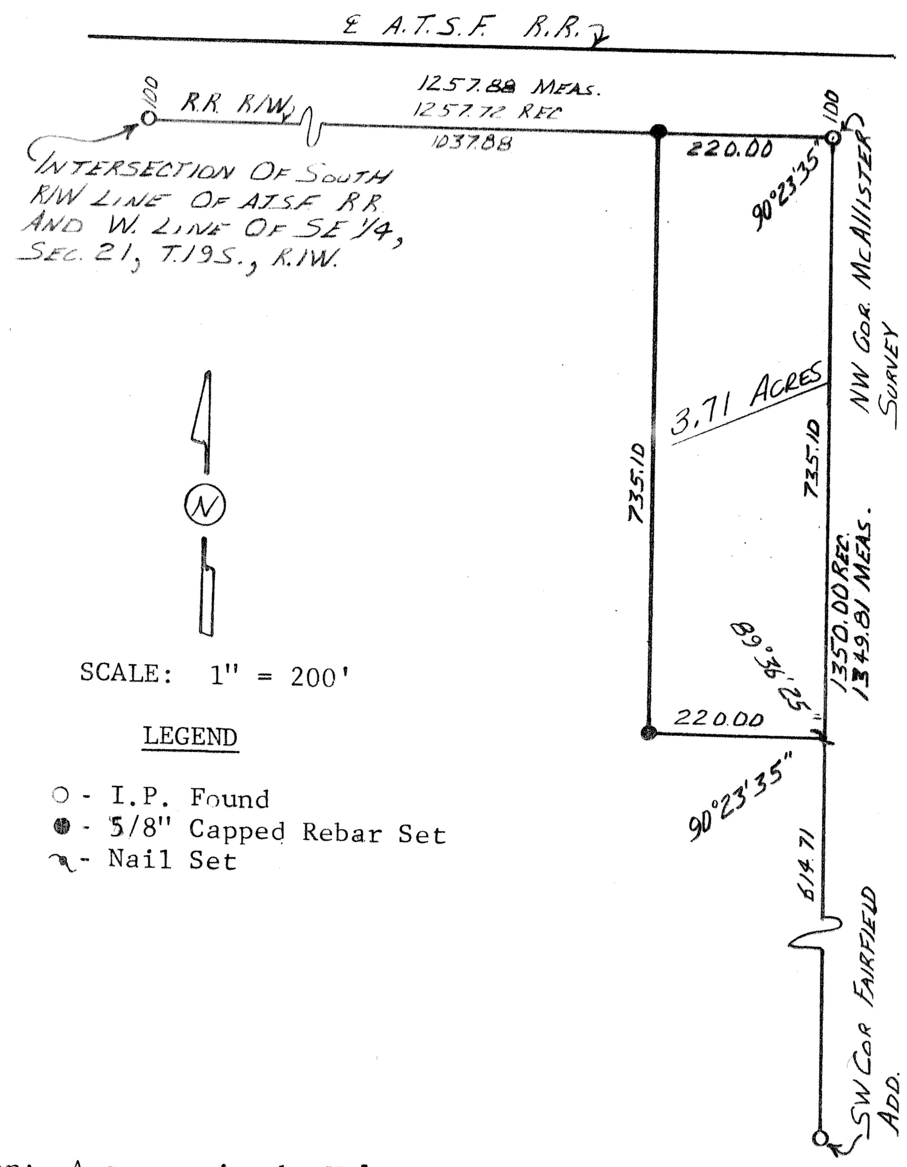
Description: A survey in the W.>, of the SE½, Sec. 21, T.19S., R.1W. of the 6th Principal Meridian, McPherson Co., Kansas as described on the attached sheet.
