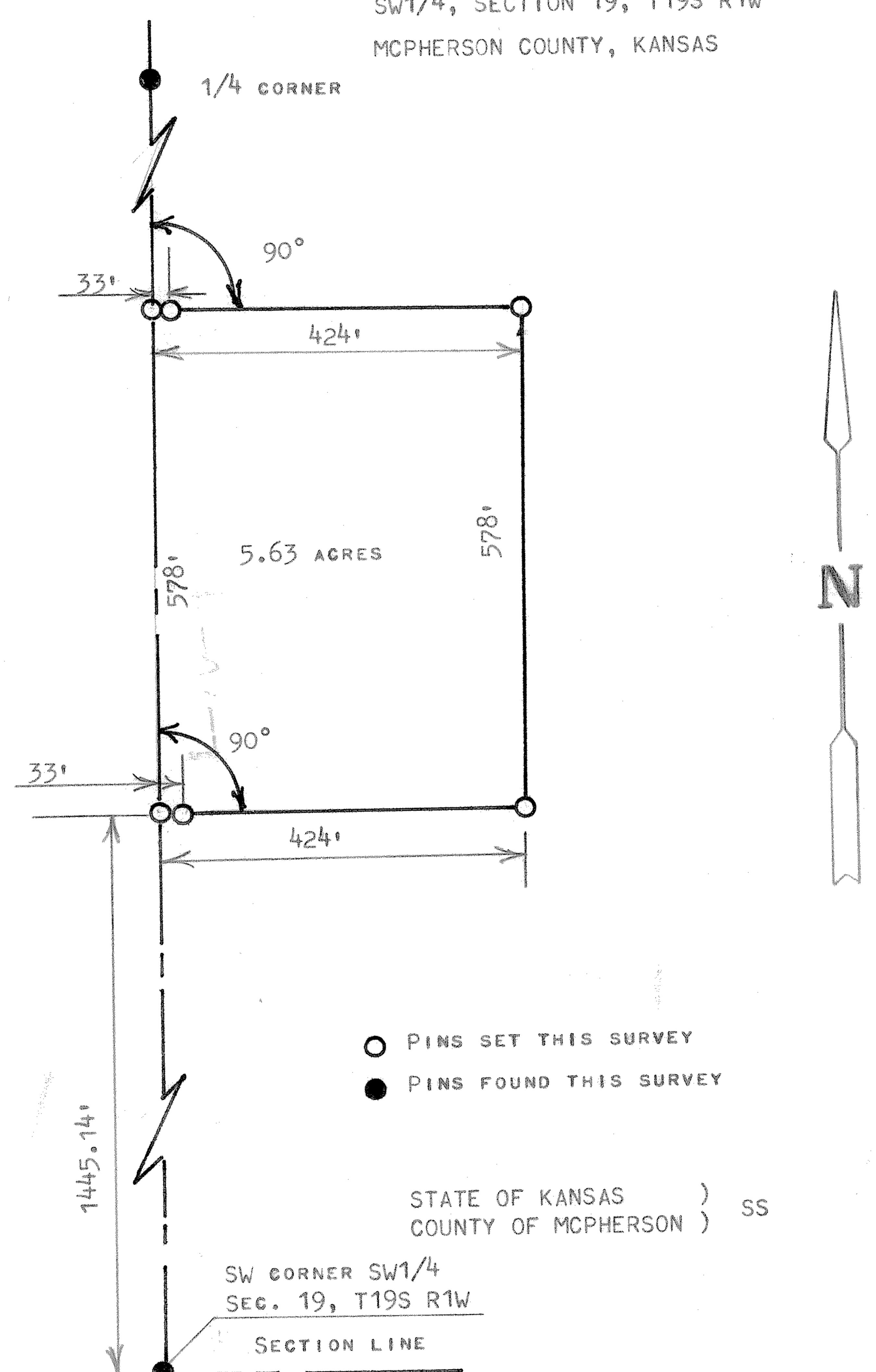
I, MELVIN FERGUSON, PROFESSIONAL ENGINEER OF THE STATE OF KANSAS DO HEREBY CERTIFY THAT UNDER MY SUPERVISION A SURVEY WAS MADE OF A TRACT OF LAND IN THE SW1/4, SECTION 19, T195 R1W of THE 6TH P.M. AND DESCRIBED AS FOLLOWS;
