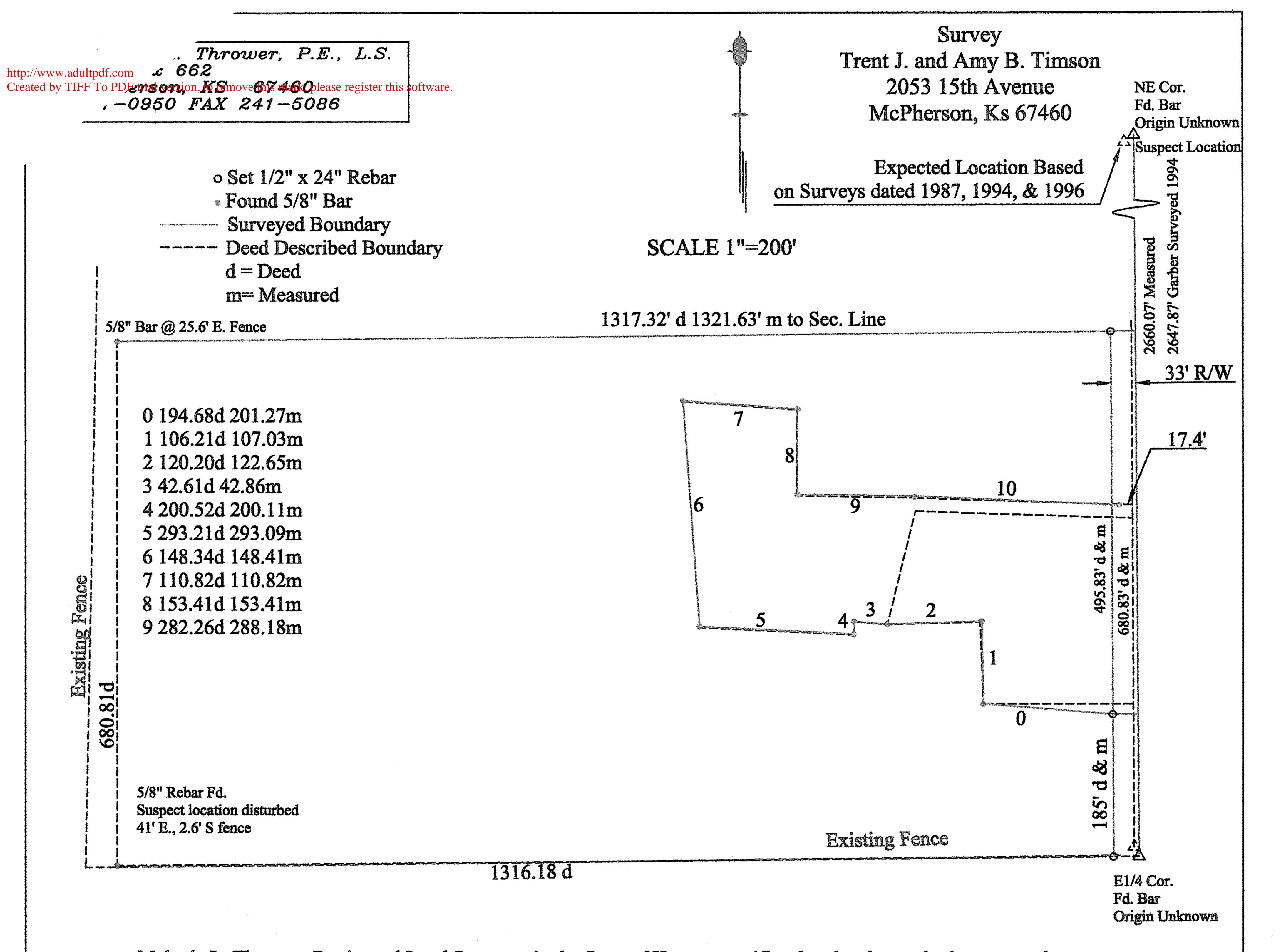
Melanie L. Thrower, Registered Land Surveyor in the State of Kansas, certifies that the above plat is a true and accurate representation of survey performed on June 27, 2001.
