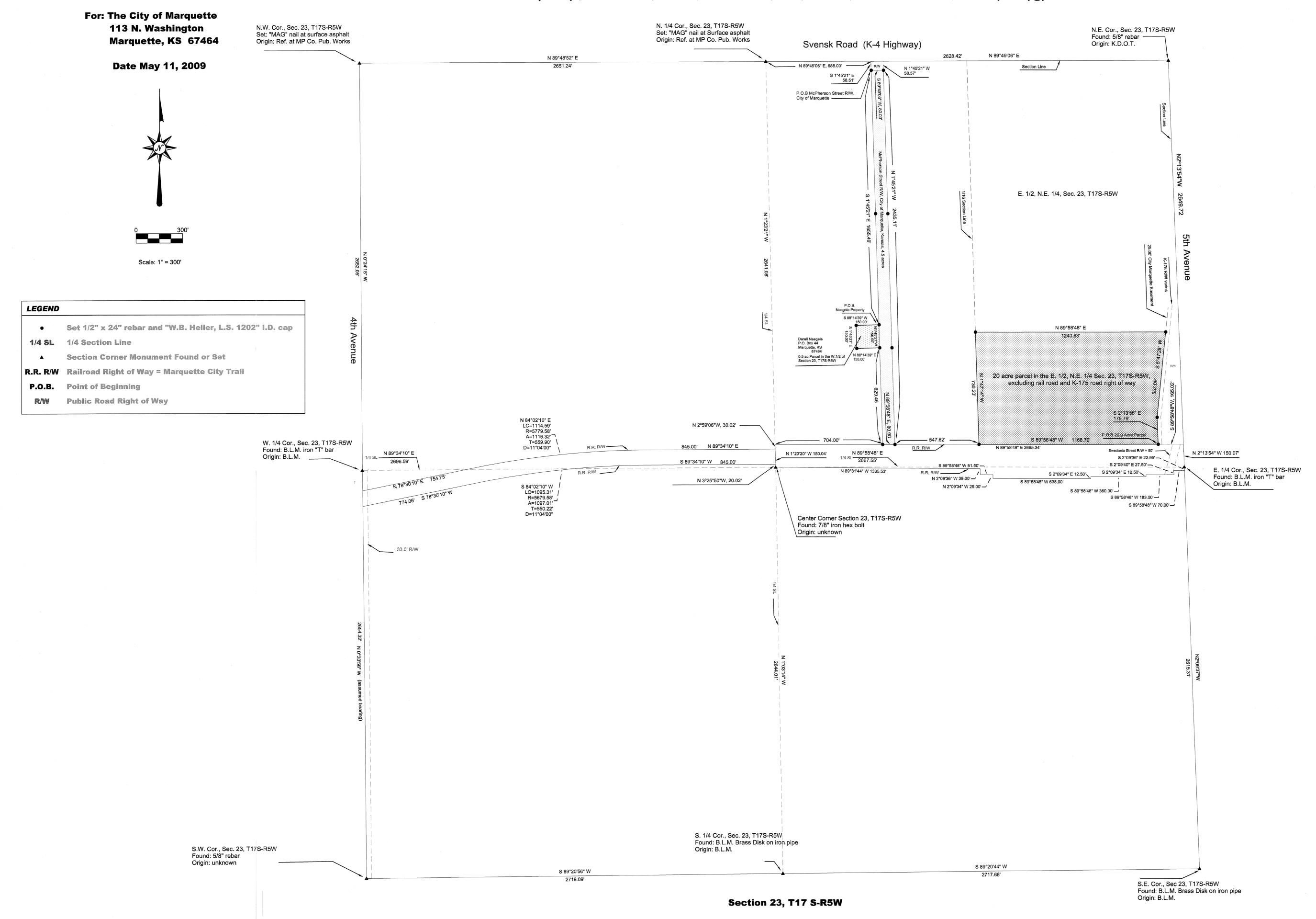
Note: All section corners and travese points were initially surveyd with G.P.S. Railroad plan information was used for the railroad was esablished by existing railroad bridge location. Deed information and G.I.S. maps from McPherson County were used to verify railroad right of way.
