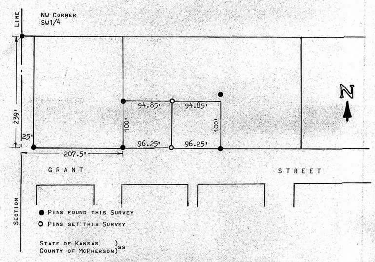
I MELVIN FERGUSON, COUNTY ENGINEER OF MCPHERSON COUNTY, KANSAS, DO HEREBY CERTIFY THAT UNDER MY SUPERVISION A SURVEY WAS MADE OF A TRACT OF LAND IN THE W1/2, SW1/4 of Section 17, T175 - R3W of the 6th P.M. and described as follows.
