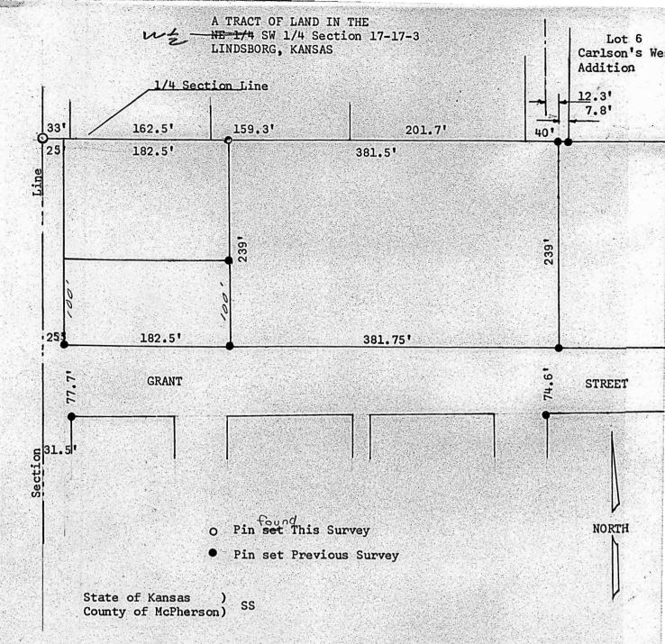
I, F. R. Rankin, County Engineer of McPherson County, Kansas, do hereby certify that under my supervision a survey was made of a tract of land in the NW 1/4, SW 1/4 Section 17, T17S, R3W of the 6th P.M.
