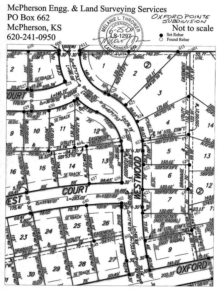
On June 25, 2004, Melanie L. Thrower set  $\frac{1}{2}$ " x 2' rebar with surveyor ID caps at locations shown in accordance with plat.
