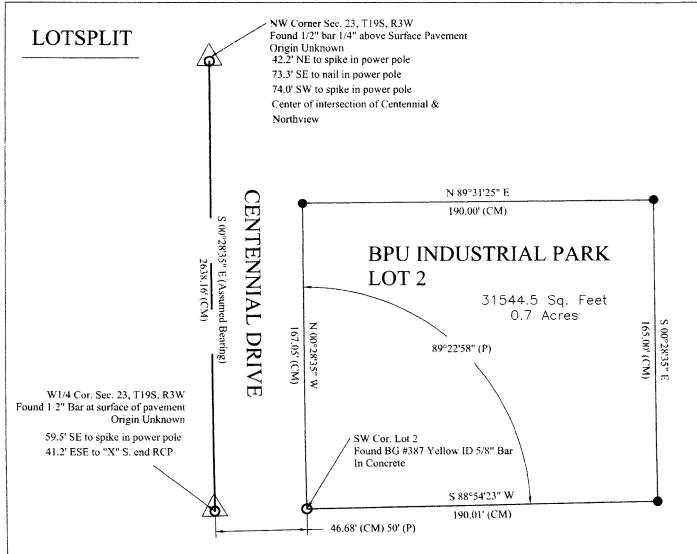
On April 27, 2012, Melanie Thrower, licensed land surveyor in the State of Kansas surveyed the following described tract of land. Tract was surveyed using Topcon GR3 GPS with grid to ground, GEOID 03, KSSOUTH.
