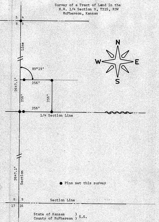
I. F. R. Rankin, Professional Engineer of the State of Kansas, do hereby certify that under my supervision a survey was made in the N.W. 1/4 Section 9 T21S, R3W of the 6th. P.M. and described as follows:
