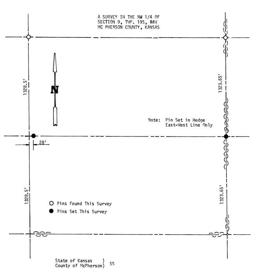
I, F. R. Rankin, County Engineer of McPherson County, Kansas, do hereby certify that under my supervision a survey was made of a line between the N1/2 and the S1/2 of the NW1/4 of Section 9, T19S, R4W of the 6th P.M. The above plat is a true exhibit of said survey as far as it is known to me.
