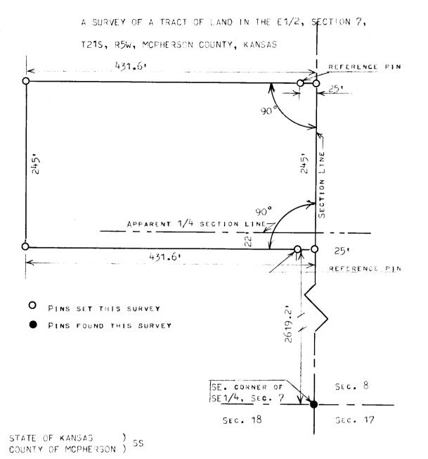
1, Melvin Ferguson, Professional Engineer of the State of Kansas do Hereby Certify that under my supervision a survey was made of a tract of Land in the E1/2, of Section 7, T215, R5W of the 6th P.M. and described as follows;
