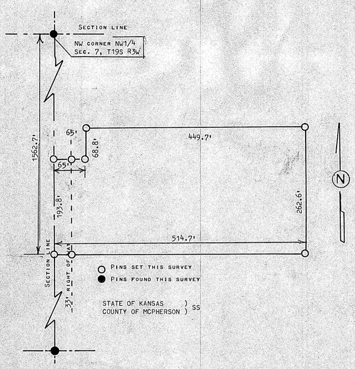
I, Melvin Ferguson, Professional Engineer of the state of Kansas do Hereby Certify that under my supervision a survey was made of a tract of Land in the NW1/4, Section 7, T195 R3W of the 6th P.M. and described as follows;
