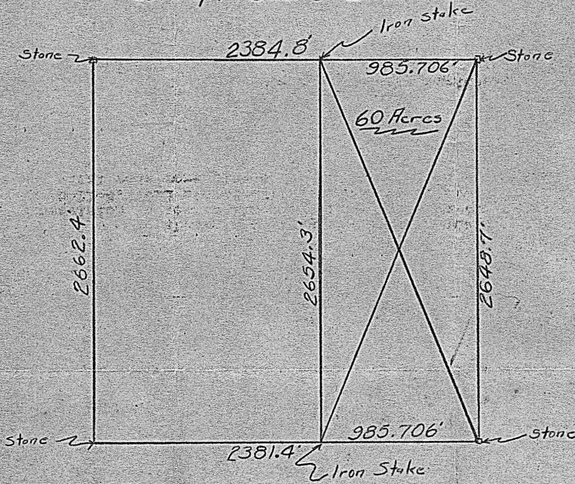
The above is a plat of a survey made under my supervision to locate the east sixty acres in the SW ~~1/4~~ <sup>1/4</sup> Sec 6-21-4. Old stones were found on the eastern boundary and steel rods were placed for the corners on the west.
