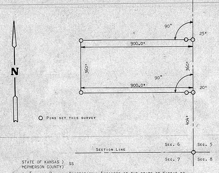
I, Francis Rankin, Professional Engineer of the State of Kansas do Hereby certify that under my supervision a survey was made of a tract of Land in the SE 1/4 Section 6, T19S R3W of the 6th P.M. and described as follows; commencint at a point 404.0 feet North of the SE corner of the SE 1/4 of Said Section 6, T19S R3W, for place of Beginning; thence Right angle West 900.0 feet; thence North Parallel with Section Line 360.0 feet; thence East to section line 900.0 feet; thence South
