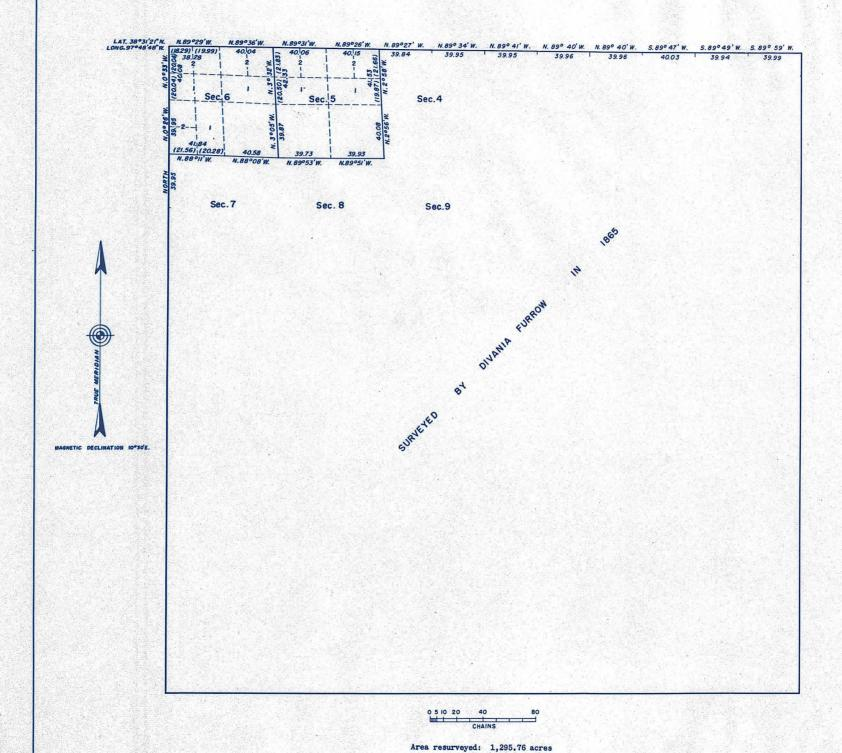
This plat represents a resurvey of a portion of the West boundary and a portion of the Subdivisional Lines of T. 18 S., R. 4 W. of the Sixth Principal Meridian, Kansas, designed to restore the corners in their original locations according to the best available evidence. The lottings and areas are as shown upon the plat of the survey approved September 19, 1865.
