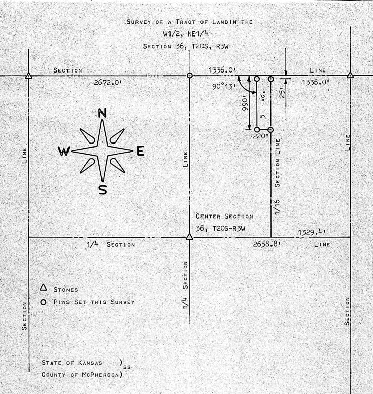
I, F. R. RANKIN, COUNTY ENGINEER OF McPherson, Kansas, do Hereby Certify that under my supervision a survey was made in the W1/2,NE1/4 of Section 36, T2OS-R3W of the 6th P.M. and described as follows;
