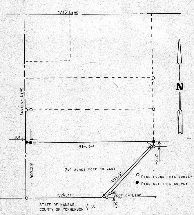
1, Melvin Ferguson, Professional Engineer of the state of Kansas do Hereby Certify that unper my supervision a survey was made of a tract of Land in the SW1/4, SW1/4, of Section 34, T198, R3W of the 6th P.M. and described as follows;
