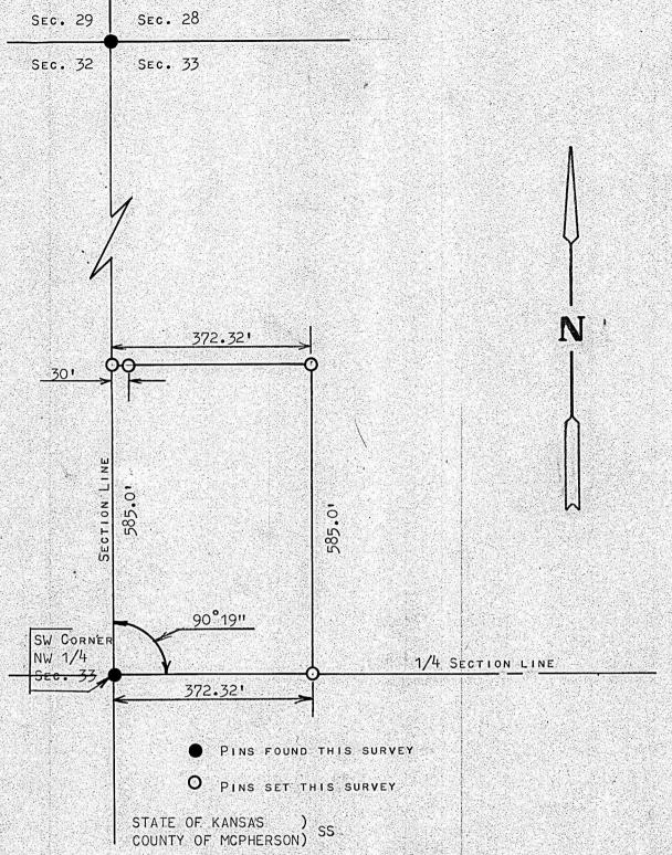
I, FRANCIS RANKIN, PROFESSIONAL ENGINEER OF THE STATE OF KANSASS DO HEREBY CERTIFY THAT UNDER MY SUPERVISION A SURVEY WAS MADE IN THE NW1/4 OF SECTION 33, T21S-R1W OF THE 6TH P.M. AND DESCRIBED AS FOLLOWS;
