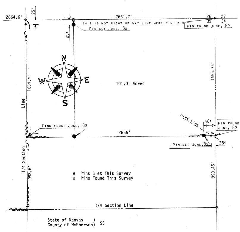
I, F. R. Rankin, County Engineer of McPherson County, Kansas, do hereby certify that under my supervision a survey was made of the N 1/2, NE 1/4 and the N 1/4, S 1/2, NE 1/4 Section 33, T20S, R4W of the 6th P.M. and the above plat is a true exhibit of said survey as far as it is known to me.
