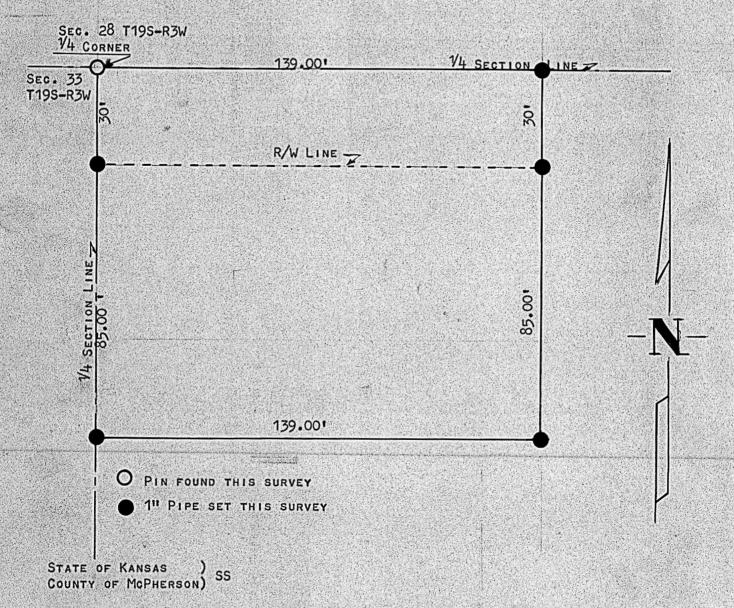
I, FRANCIS D. WAGNER, COUNTY ENGINEER OF MCPHERSON COUNTY, DO HEREBY CERTIFY THAT I DID CAUSE TO BE DONE ON THE 7TH DAY OF JUNE, 1961 A SURVEY OF A TRACT OF LAND IN THE NWV4 OF THE NEW 4 SECTION 33, T19S-R3W OF THE 6TH P. M. AND DESCRIBED AS FOLLOWS:
