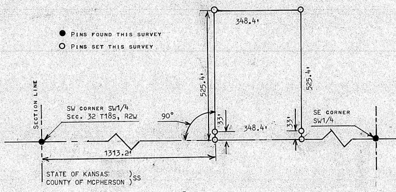
I, MELVIN FERGUSON, PROFESSIONAL ENGINEER OF THE STATE OF KANSAS DO HEREBY certify that under my supervision a survey was made in the SW1/4, Section 32, T18S R2W of the 6th P.M. and described as follows;
