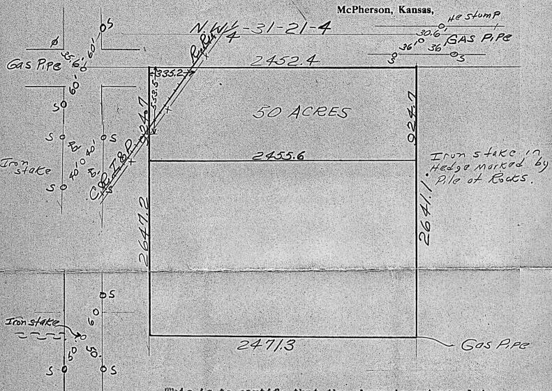
This is to certify that the above is a true plat of a survey made by me March 22, 1935, for G / Toevs to locate the north fifty acres of the NV of Sec 31-21-4, said fifty acres to be exclusive of the railroad right of way and the tract lying north and west of the railrod. The corners are marked as shown above.
