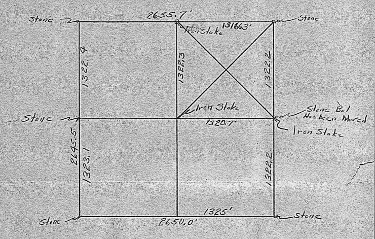
The above is a plat of a survey made under my supervision for C M Toevs to locate the NE  $\frac{1}{4}$  SW  $\frac{1}{4}$  Sec 30-20-4. The old stone at the center of the section was found and a stone placed by Bert Rowland at the SE Cor of the forty was also found but this had evidently been moved so a steel rod was placed at the correct location. Steel rods were placed at the two corners on the west.
