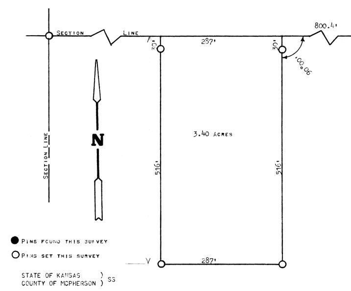
I, Francis Rankin, County Engineer of McPherson County, Kansas, do Hereby certify that under my supervision a survey was made of a tract of Land in the NW  $^{74}$  of Section 30, T17S-R4W of the 6th P.M., and described as follows:
