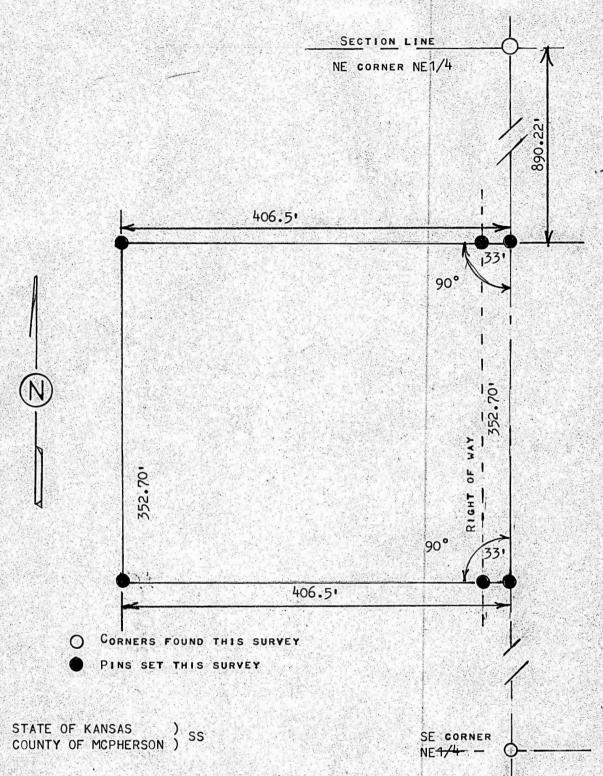
1, Melvin Ferguson, Professional Engineer of the state of Kansas do hereby Certify that under my supervision a survey was made in NE1/4, Section 3, T19S, R4W of the 6th P.M. and described as follows;
