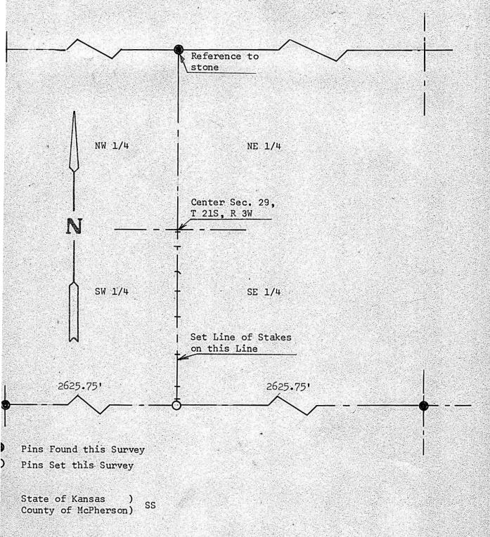
, F. R. Rankin, County Engineer of McPherson County, Kansas, do hereby certify hat under my supervision a survey was made to determine the 1/4 section line etween the SW 1/4 & SE 1/4 of Section 29, T 21S, R 3W of the 6th P.M. and that ne accompanying plat is a true exhibit of said survey as far as it is known to
