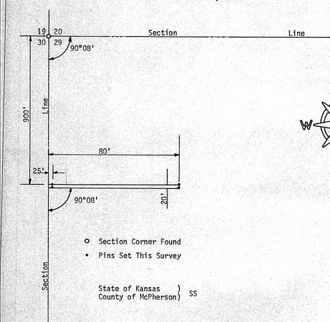
I, F. R. Rankin, County Engineer of McPherson County, Kansas, do hereby certify that under my supervision a survey was made in the NW 1/4 of Section 29, T19S, R4W of the 6th P.M. and described as follows:
