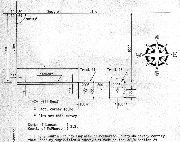
I F.R. Rankin, County Engineer of McPherson County do hereby certify that under my supervision a survey was made in the NW1/4 Section 29 T19S, R4W of the 6th P.M. And described as follows:
