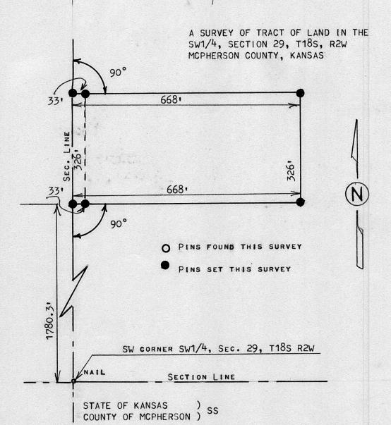
I, MELVIN FERGUSON, PROFESSIONAL ENGINEER OF THE STATE OF KANSAS DO HEREBY CERTIFY THAT A SURVEY WAS MADE OF TRACT OF LAND IN THE SW1/4, SECTION 29, T18S, R2W OF THE 6TH P.M. AND BESCRIBED AS FOLLOWS;
