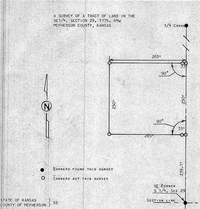
, Melvin Ferguson, Professional Engineer of the state of Kansas do Hereby CERTIFY THAT UNDER MY SUPERVISION A SURVEY WAS MADE IN THE SE1/4, Section 29, T17S, R4W of the 6th P.M. and described as follows:
