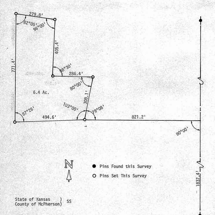
I, Melvin Ferguson, County Engineer of McPherson County, Kansas do hereby certify that under my supervision a survey was made of a tract of land in the E1/2, SE1/4 of Section 28, T17S, R5W of the 6th P.M. and described as follows:
