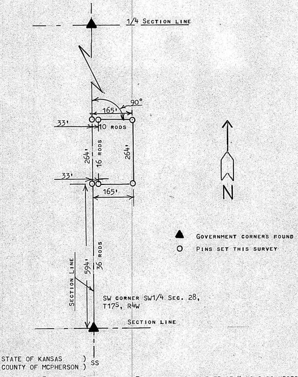
1, Melvin Ferguson, Professional Engineer of the State of Kansas do Hereby Certify that under my supervision a survey was made of a tract of Land in the SW1/4, Section 28, T17S R4W of the 6th P.M. and described as follows:
