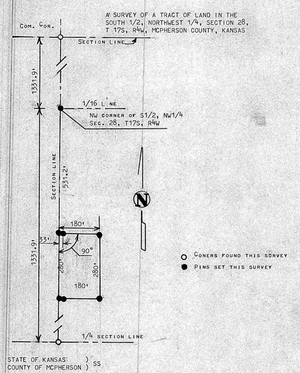
I, Melvin Ferguson, Professional Engineer of the state of Kansas do Hereby Certify that under my supervision a survey was made under my supervision of a tract of Land in the S1/2,NW1/4, Section 28, T17S, R4W of the 6th P.M. and described as follows;
