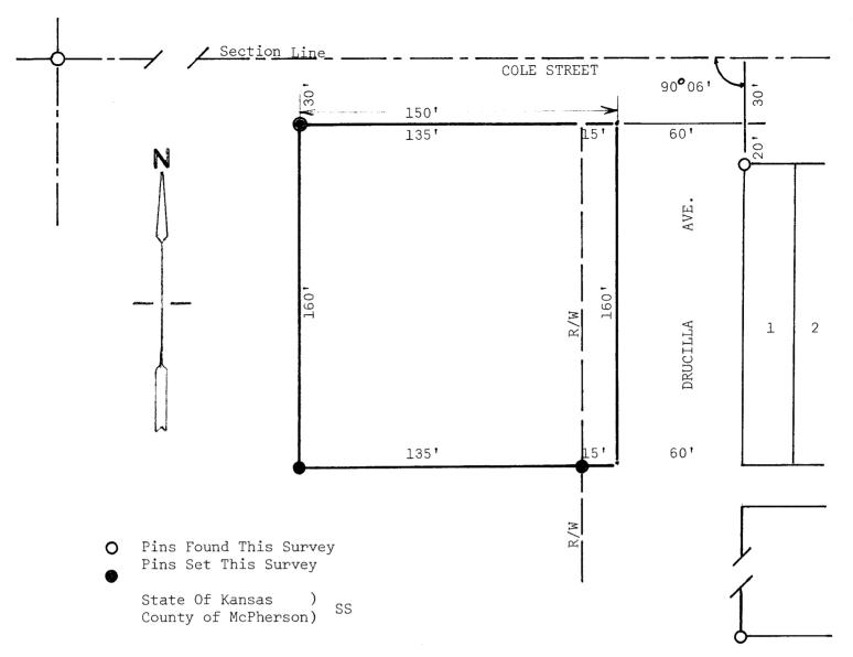
I, Melvin Ferguson, County Engineer of McPherson County, Kansas, do hereby certify that under my supervision a survey was made in the  $W^1_{\geq}$  of the NE $^1_{\leq}$  of Section 27, T21S, R2W of the 6th P.M. and described as follows:
