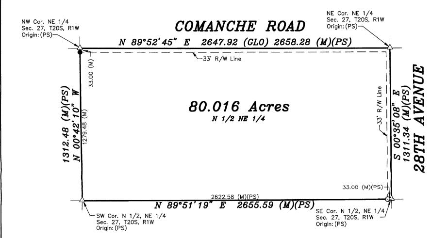
**LEGEND** Sectional Monument Fd. 5/8" Rebar w/GSS CLS 52 Cap ⊙ - Fd. 5/8" Rebar w/GSS CLS 52 Cap 5/8" x 24" Iron Rebar Set w/GSS CLS 52 Cap NOR Measured General Land Office GLO — (PS) - Previous Survey GSS Project #G2015-161 Scale: 1"= 400' BASIS OF BEARING
