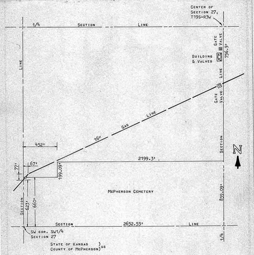
I, Melvin Ferguson, County Engineer of McPherson County, Kansas, do hereby certify that under my supervision a survey was made in the SW1/4 of Section 27, T19S-R3W of the 6th P.M., of a Gas Line Easement \_\_\_\_\_ feet on each side of a line described as follows:
