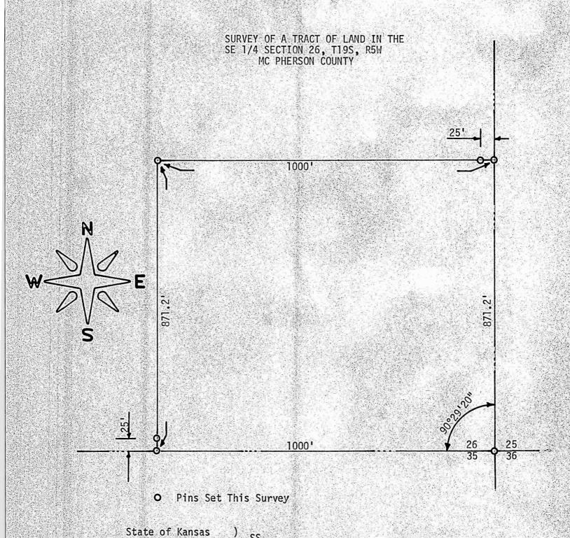
I, F. R. Rankin, County Engineer of McPherson, Kansas, do hereby certify that under my supervision a survey was made in the SE 1/4 Section 26, T19S, R5W of the 6th P.M. and described as follows:
